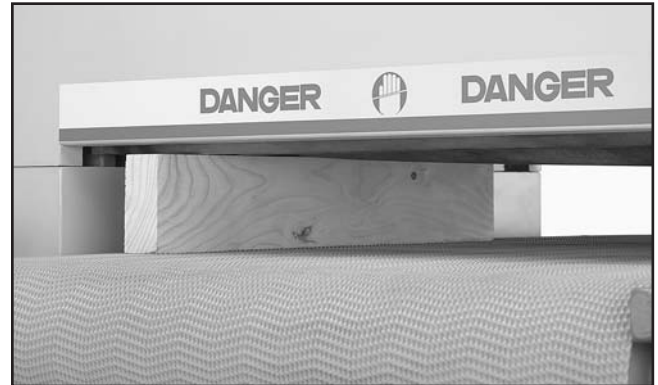
Figure 20. Checking pressure roller height.
